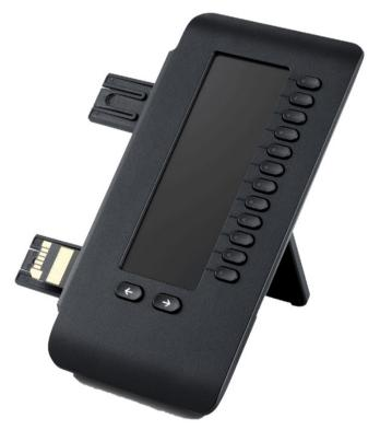
The diagram shows the OpenScape Key Module 600. You can attach up to two OpenScape Key Module 600s to OpenScape Desk Phone CP700 and up to four OpenScape Key Module 600s to OpenScape Desk Phone CP700X.
