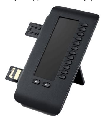
The diagram shows the OpenScape Key Module 600. You can attach up to two OpenScape Key Module 600 to OpenScape Desk Phone CP700 and up to two OpenScape Key Module 600s to OpenScape Desk Phone CP700X.
