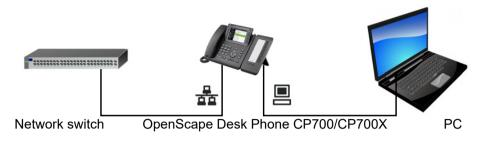
Using this connection option saves one network port for each switch used and requires shorter network cables.
