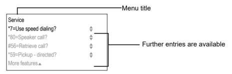
The menu structure consists of two levels. The first line in this structure shows the menu currently selected while the remaining lines show the options for this menu. The arrow next to an entry indicates the availability of additional options for this entry.
