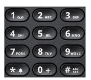
You can only use the digits 1 to 9 and 0 as well as the \* and # characters when dialing a number. Press to delete digits (only if en-bloc dialing is enabled).
