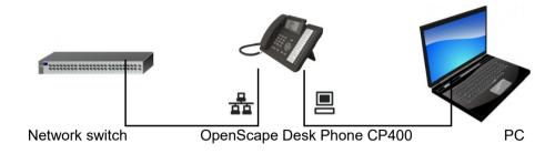
Using this connection option saves a network port for the switch used and allows shorter network cables to be used.
