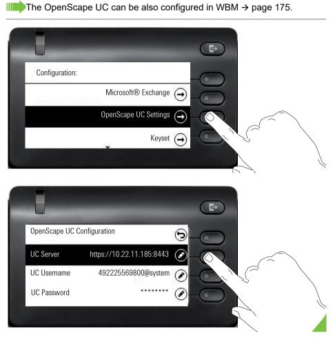
The OpenScape CP400 will login using the given user credentials. If the data is incomplete (missing server address, username or password) the phone will not try to login at all.
