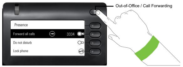
Personal Presence via the phone is temporarily suspended by means of call forwarding or do not disturb.
