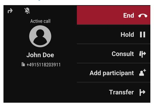
During a call, select any function key to perform the corresponding action such transferring the call.
