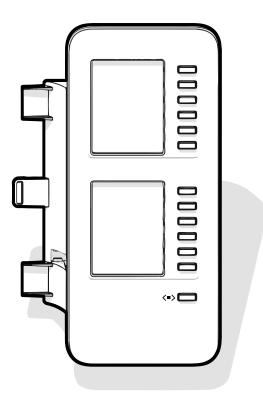
The KM710 is an optional key module attached and connected to the right side of the phone that provides an additional 12 illuminated and programmable function keys at two levels, i.e. additional 24 functions (see "Programmable function keys"  $\rightarrow$  page 60).
