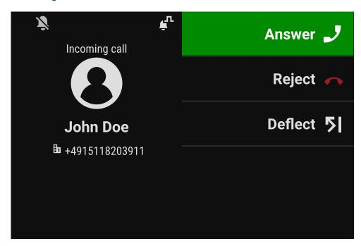
Your phone rings and the notification LED flashes. In addition to the common phone functions such as "Accept", additional information and functions may be displayed.
