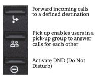
Forward, Pick up and DND are default settings and can be programmed with different functions.
