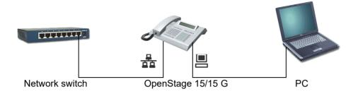
Using this connection option saves one network port for each switch used and requires fewer or shorter network cables when arranged correctly.
