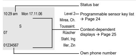
The left area contains the status bar on the first line and is followed by a five-line field for comprehensive context-specific displays. The right area is used for labeling the programmable sensor keys.
